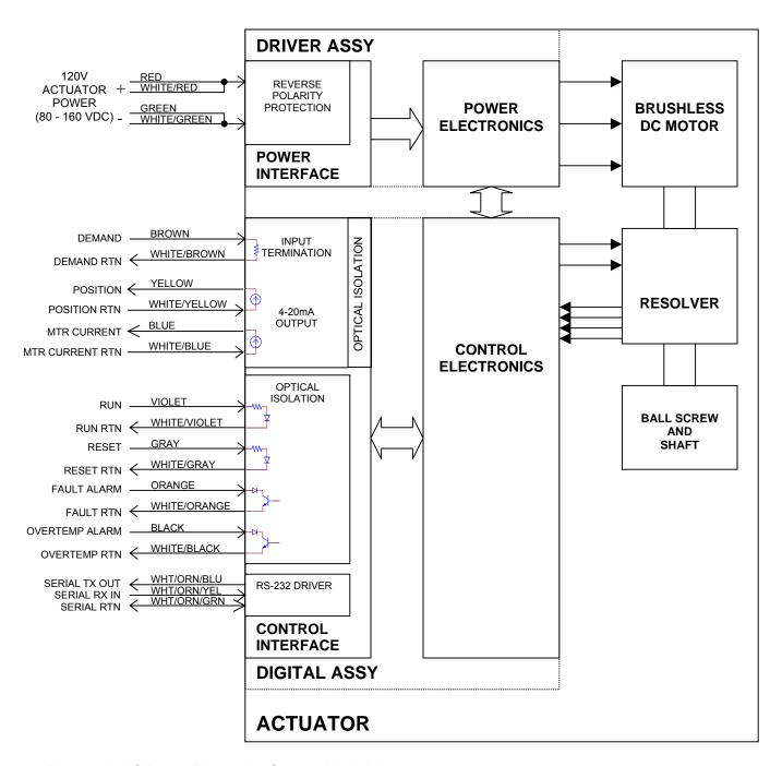
Figure 2-1: ACT2000 Electronics System Block Diagram
